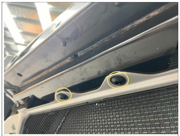
31. Remove the 2x T30 Screws holding the bash plate to the center crossbeam.
