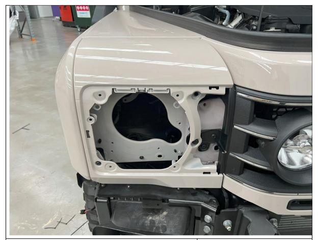
100. Temporarily re-fit the headlight surround panel, to allow reference for alignment of bar.
