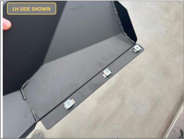
139. Fit 3x M6x2mm Cage nuts to each of the side under panels.
