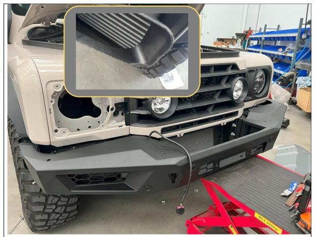
102. With assistance, either from another person, or a lifting trolley, lift the bar onto the mounts on the vehicle.
