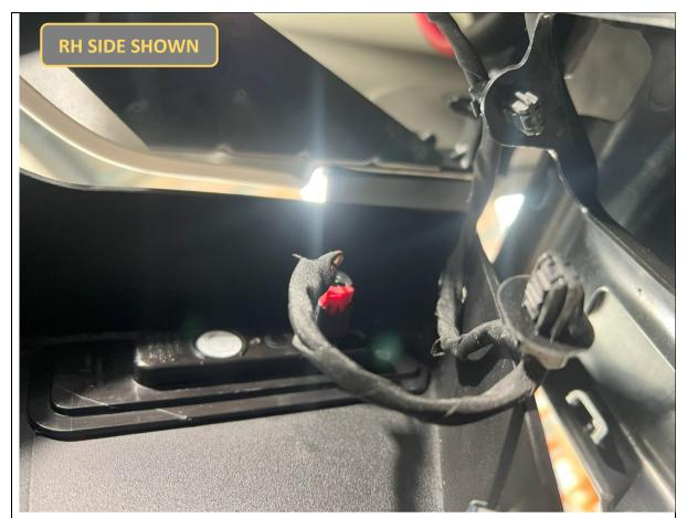
120. From underneath, reconnect the side clearance lamp electrical connectors.
