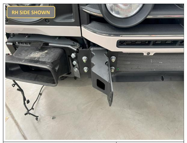
39. Secure the impact assembly to the chassis and auxiliary radiator bracket, re-using the factory bolts and flange nuts removed from the impact beam.
