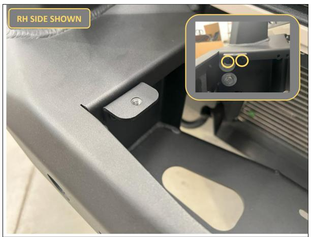
109. If NOT fitting a winch, fit the winch cover panel brackets to the bar using M6x16 button head bolts, Flat washers and flange nuts supplied with the winch cover kit.
