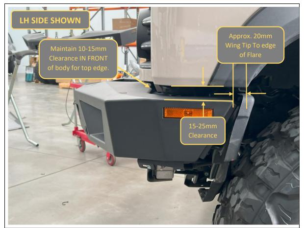
106. With assistance from another person, Align the bar with the edges of the vehicle. Adjust such that the clearances are neat and even side to side.
