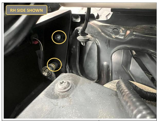
127. Once the inner arch bracket is connected, tighten the M6 bolts securing the bracket to the wing, using 10mm socket or spanner
