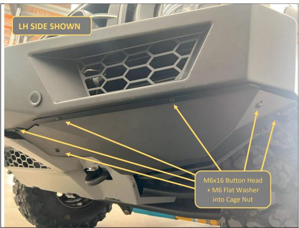
143. Fit Side Under panels using 6x M6x16 button head bolts and flat washers into the cage nuts placed earlier.
