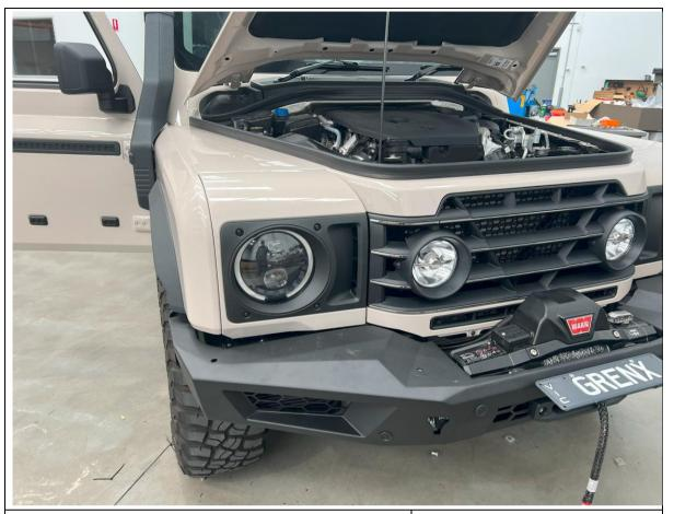
132. Replace the headlight and all trims on the RH front headlight, re using all original fasteners.
