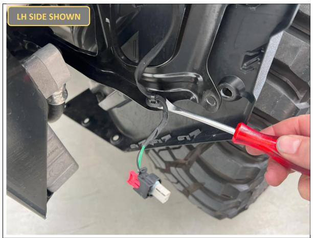
29. Unclip the clearance light harness from the wheel arch bracket.
